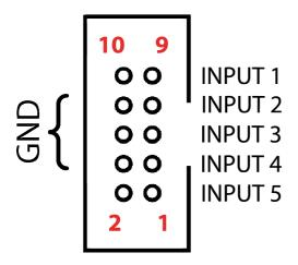
This connector provides input for user-assigned functions.
