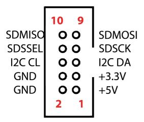
This connector allows use of SD Card with Planet-CNC SD card adapter and I2C protocol devices. An inexpensive I2C LCD digital readout has been successfully prototyped, tested and documented.
