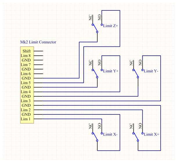
Each limit switch is connected to its own input limit pin.
