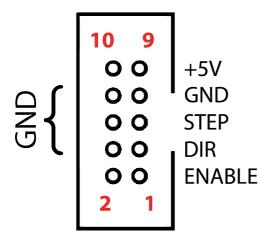
Each connector controls one motor driver. Controller has 4 connectors for axes 1-4. Axes 5-9 use common connector described in next chapter. In total this means 9 axes which all can be moved at same time.
