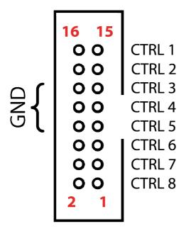
This connector provides inputs for use of MPG pendant devices and E-Stop. Spindle speed encoder for spindle synchronization can also be connected. GND pins provide 'Ground' or common connections.
