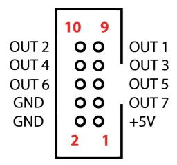
This connector provides 7 digital outputs for control of external devices. The optional 'Output board' links to the Mk2 controller using this connector. Output assignment is controlled in software.
