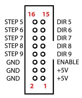
This connector controls up to 5 motor drivers. It can also provide an ENABLE signal to motor drivers that can take advantage of these feature.
