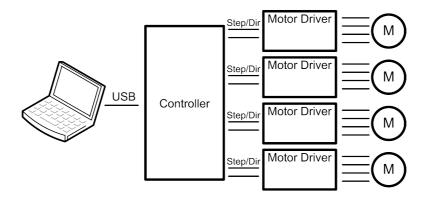
The PlanetCNC series of USB CNC motion controllers link between a personal computer and motor drivers supporting step/direction control. They are compatible with most drivers. The controllers use the USB port, available on all modern computers and laptops. They can serve as direct replacement or upgrade for many parallel port break-out boards.
