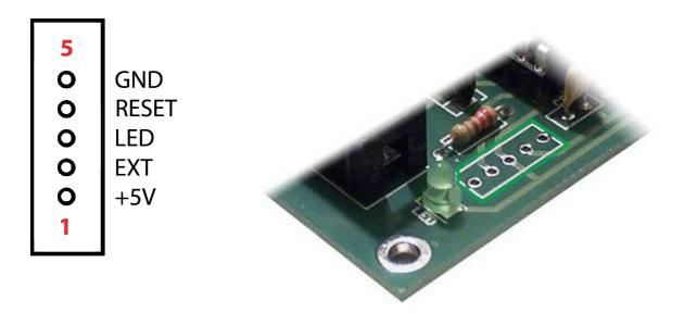
**GND:** Ground or 'common' connections.
