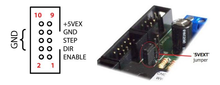
Each connector controls one motor driver.
